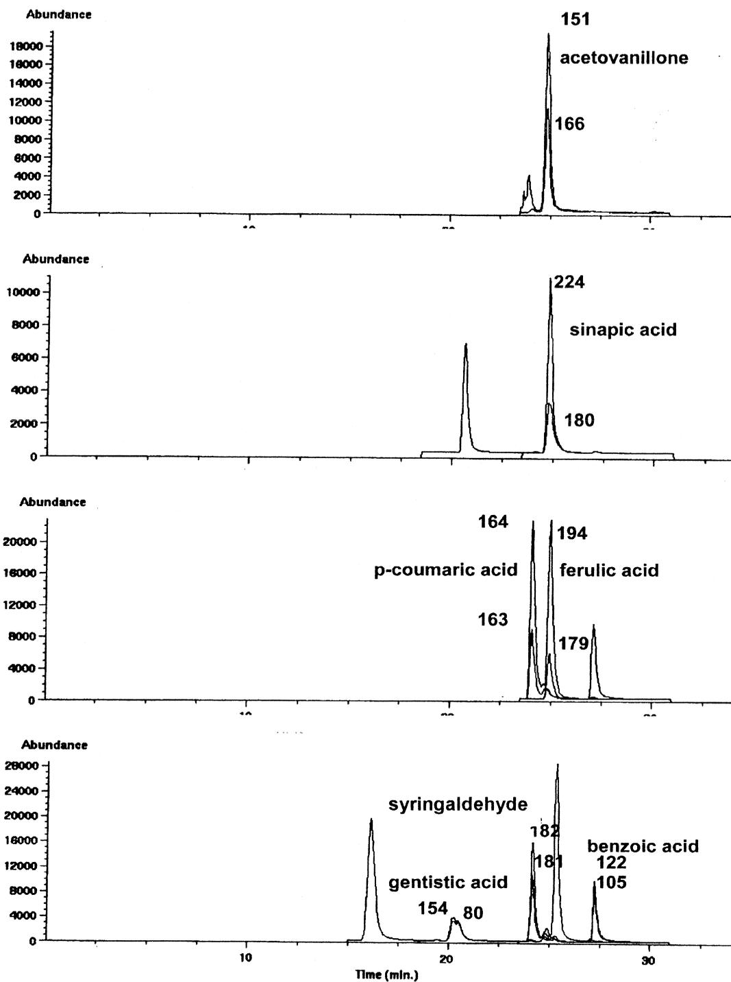
Fig. 1. Ion current profiles relative to a 0.5- $\mu$ l injection of 100 ng of phenolic compounds. Chromatographic conditions: capillary  $C_{18}$  column; mobile phase, water–acetonitrile; gradient, from 100 to 20% water in 40 min; flow-rate 1  $\mu$ l/min.
