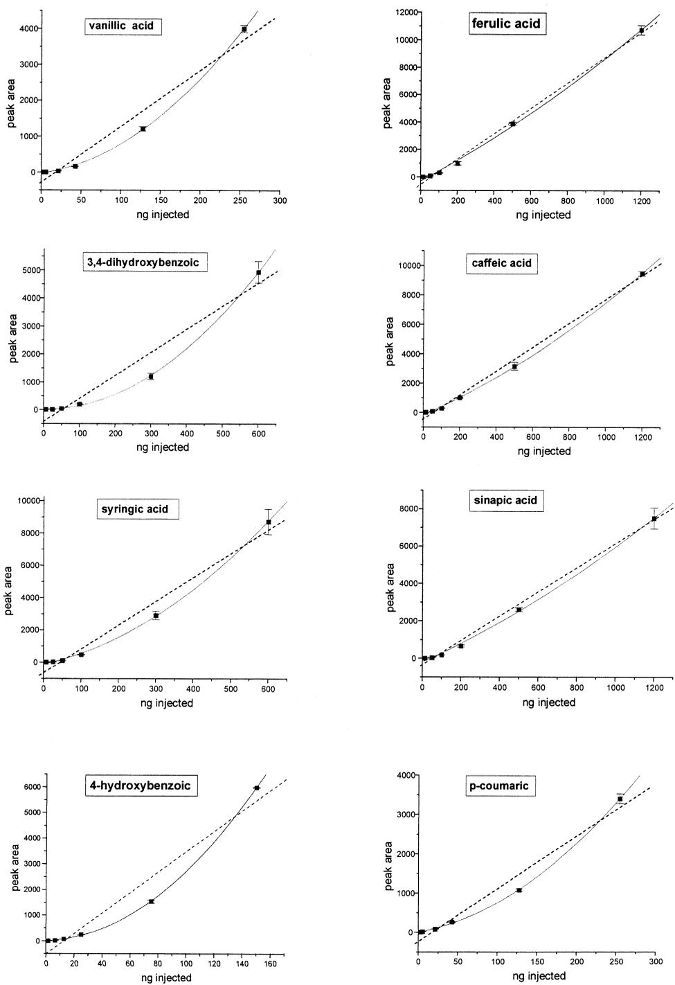
Fig. 3. Calibration graphs for selected phenolic acids. Linear and quadratic regression are reported (see text for HPLC- $\mu$ PB-MS conditions).
